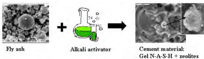
Fig.2.6 Alkali activation of fly ash
