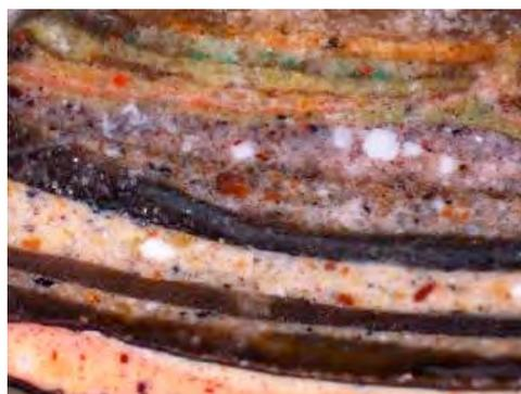
Fig.2.15. Cross section from paint sample that shows the layered structure and their heterogeneous mixtures.
