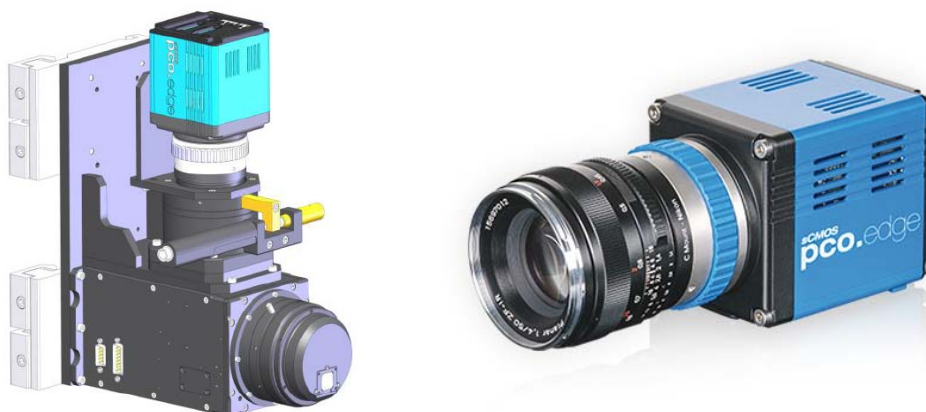
Figure 52. Left: 3D rendering of the monochromatic beam microscope mounting a PCO. Edge 4.2 camera on top. Right: photograph of a PCO. Edge 4.2
