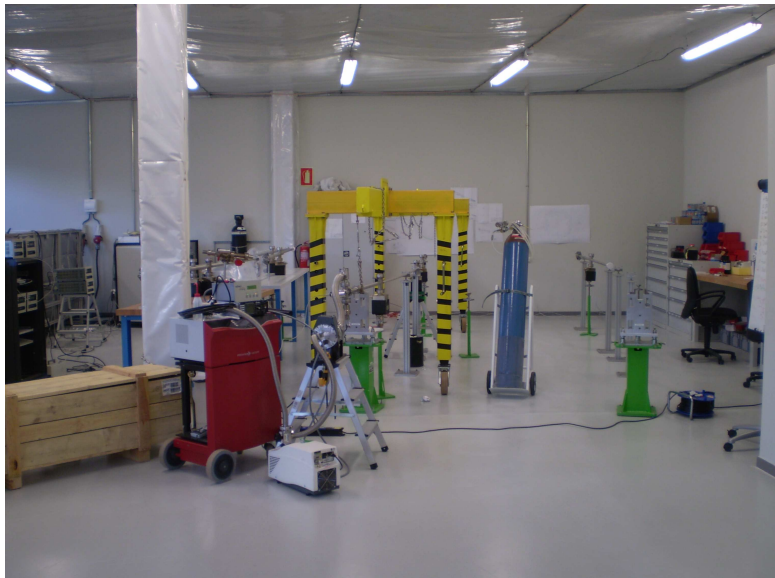
Fig.8: View of the vacuum laboratory located at the external perimeter of the building. The vacuum chambers of the booster are pumped down, baked and leak tested to prepare them for mounting in the tunnel. Date: 2 Dec 08
