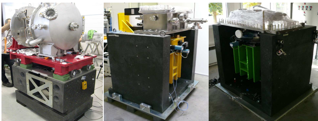
Fig.44: Main optical components of XALOC beamline. From left to right, monochromator, vertical focusing mirror (VFM) and horizontal focusing mirror (HFM).
