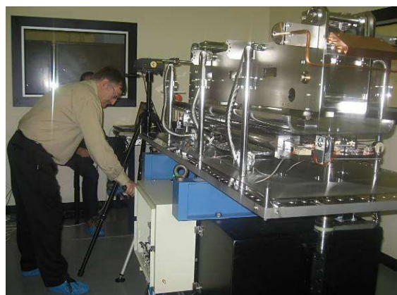
Figure 46 and 47: C. Ruget and J. Nicolas from ALBA are testing the mechanics of the monochromator (left) and collimating mirror (right).
