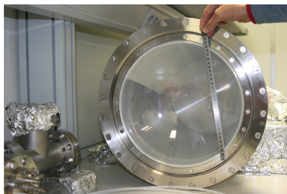
Fig. 43: The mylar vacuum to air window mounted on the end tube of the X-ray camera.
