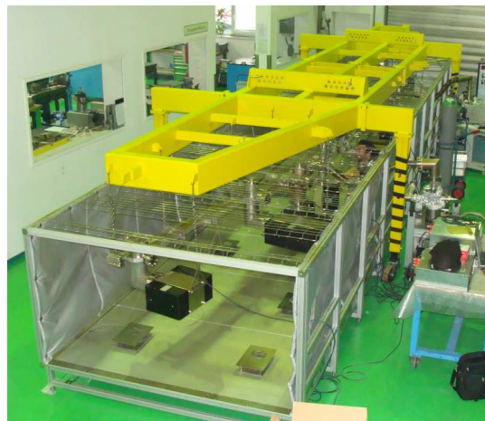
Fig.24: factory acceptance tests of the storage ring vacuum chambers, the bakeout oven and the strong back.
