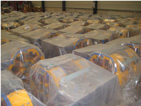
Fig. 16: View of the SR quadrupoles and sextupoles stored in the ALBA warehouse and waiting for installation.
