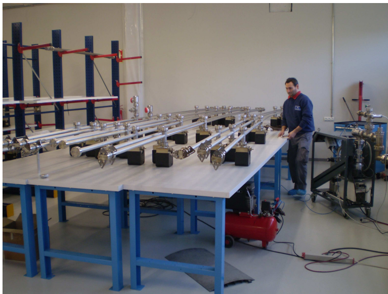
Fig.9 Several vacuum chambers tested and ready for mounting.
