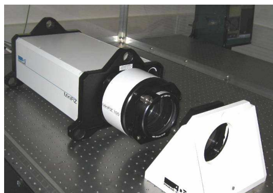
Fig.52: Picture of the Fizeau interferometer that will be used to measure the slope error of the mirrors of the first beamlines at Alba.
