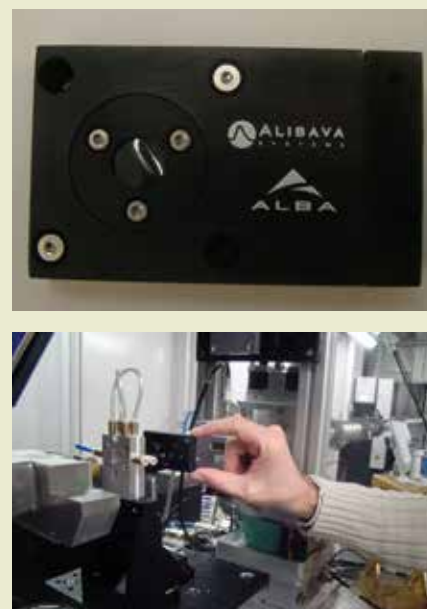
Top, photograph of the X-ray detector. Bottom, view of the detector being placed at the NCD beamline. © ALBA
