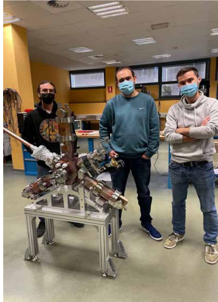
Figure 21: 3rd Harmonic Cavity Prototype at the ALBA lab with part of the RF team.
