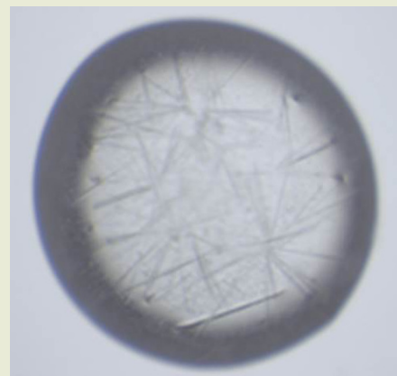
Crystals obtained in crystallization plates by using the vapour diffusion method in sitting drops. © Artax Biopharma
