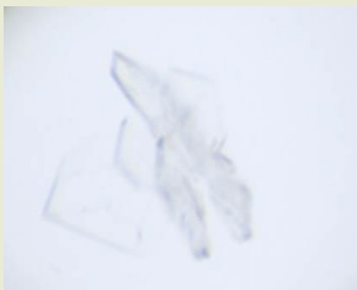
Crystals obtained in crystallization plates by using the vapour diffusion method in sitting drops. © Artax Biopharma
