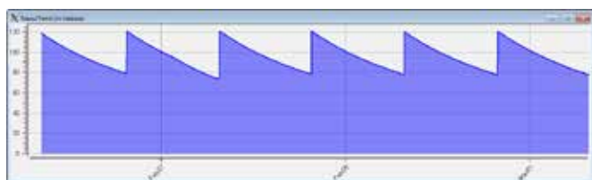
Figure 4a: Current in the SR as a function of time when operated in decay mode.
