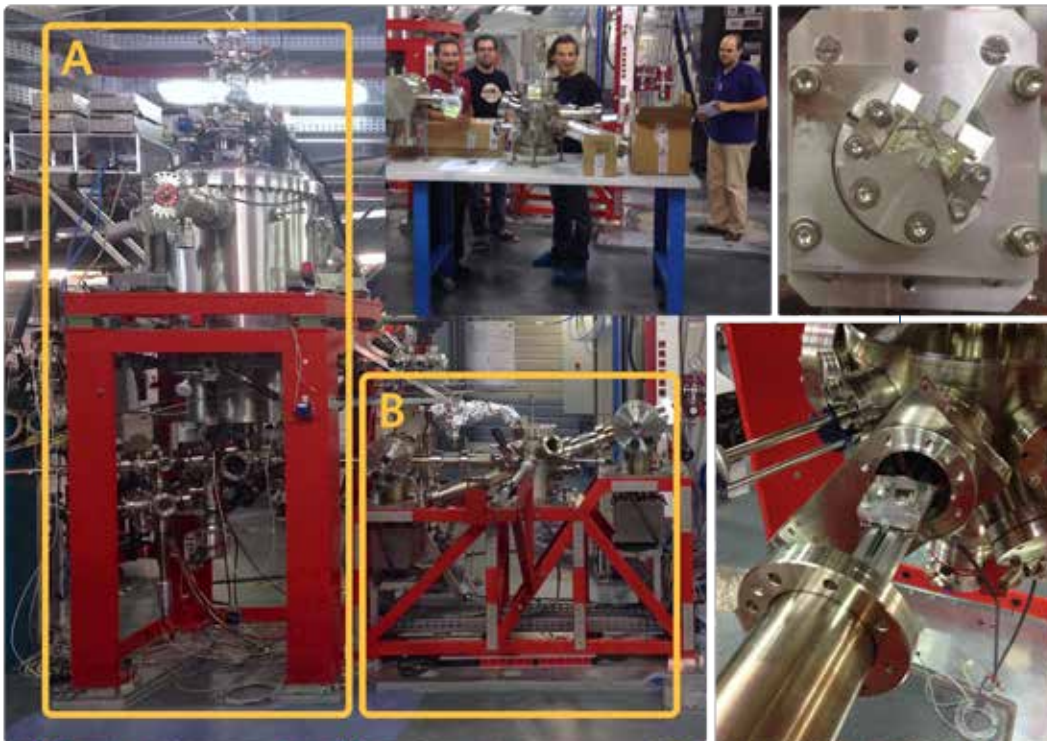
Figure 19: Boreas beamline after the SPTR installation: A) HECTOR vector magnet with preparation chamber, B) SPTR system. Right side panels: on top, a picture taken during installation and a close-up of the transfer carriage with the STM plate placed inside; beneath, the rack with the traveler entering the HECTOR preparation chamber.
