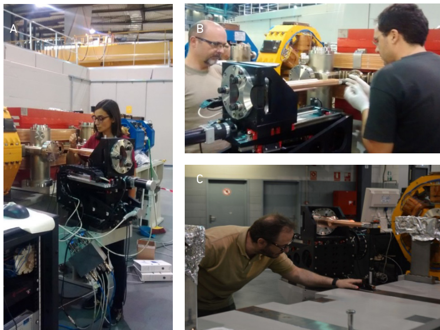
Figure 15: Assembly of the first extraction mirror mechanics. (a) Alignment procedures, (b) Motors functionality tests, (c) Metrology, Motors repeatability and Vibration tests
