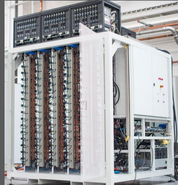
80 kW SSA for SESAME (10 dissipaters x 16 mod)
