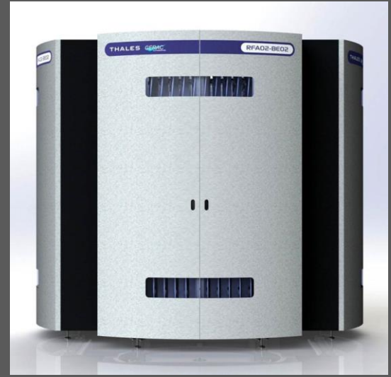
140 kW SSPA from THALES 80 : 1 cavity combiner 80 x 2 kW RF units 2 transistors per unit First demonstrator delivery in Autumn 2016
