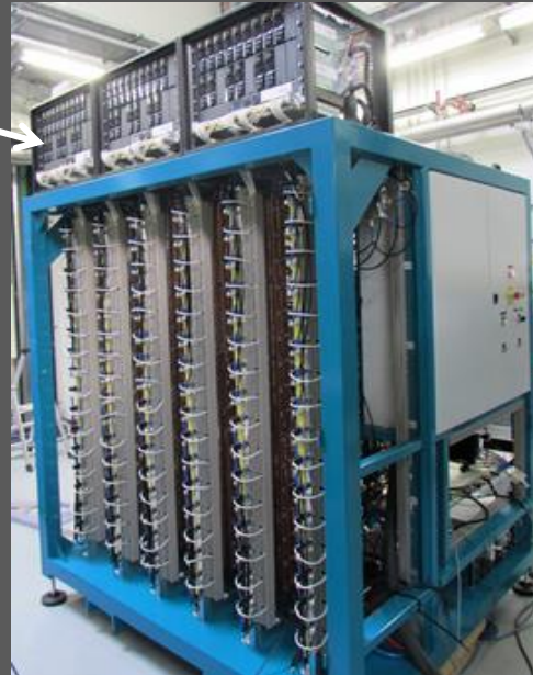
50 kW SSA for ThomX (6 dissipaters x 16 mod)
