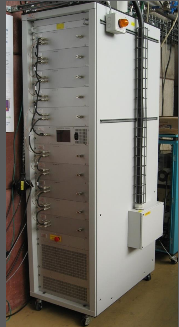
16 kW - 1.3 GHz SSPA from SIGMAPHI ELECTRONICS
