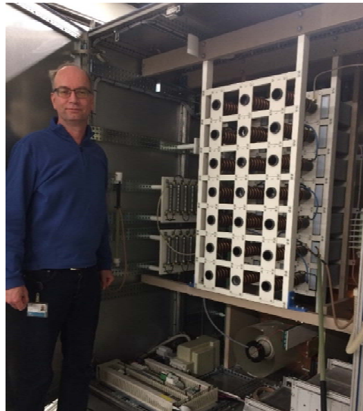
Pulse forming network 525 nF, 21.5 mH
