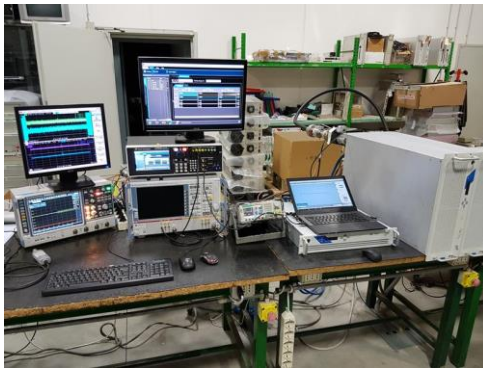
10 kW – tetrode driver - test bench
